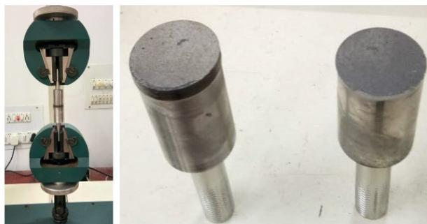
**Figure 4.** Plasma spraying torch and adhesion test set-up as per ASTM C-633 standard.
